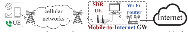
Figure 12: Exploiting the E2E communication to enable free data service using a Mobile-to-Internet gateway.
